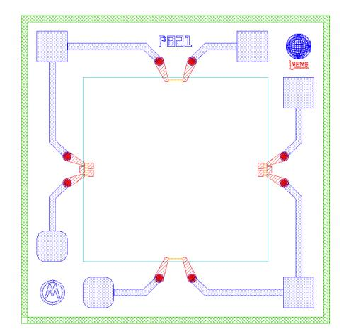
2.5mm x 2.5mm x 1mm 0.25 mm Bond Pads Pad coordinates available on Request Metallization Options for open, closed, or 2 Half Bridges are available
